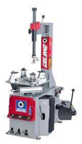
Semi-automatic swing arm tyre fitting machine for motorcycles, scooters & ATV tyres
